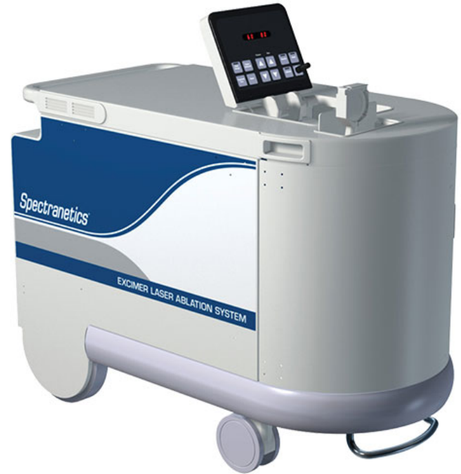
CVX-300 Excimer Laser (Spectranetics). "cold" laser operating in the ultraviolet wavelength (308 nm) The mechanism of action is photo ablation, using light to break down molecular bonds thereby vaporizing and fragmenting tissues to molecules.
